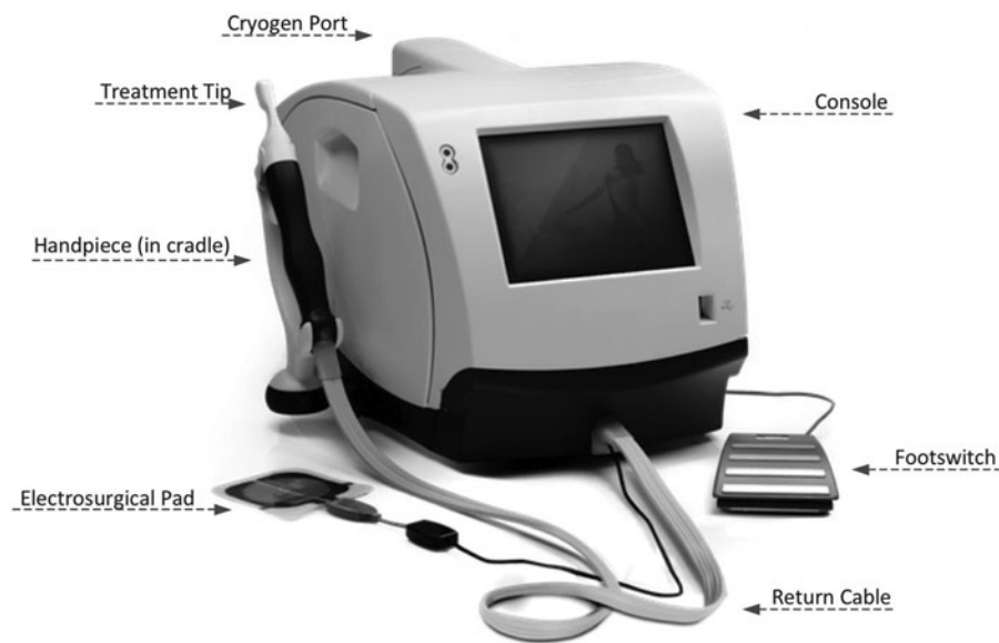
FIG. 1. The in-office procedure, table top radiofrequency (RF) system comprising a RF console with an integrated cooling module, a horizontal handpiece, and disposable, single-use treatment tip.
